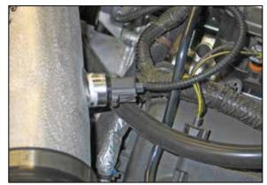
23. Connect the inlet air temperature sensor extension barness into the factory electrical
