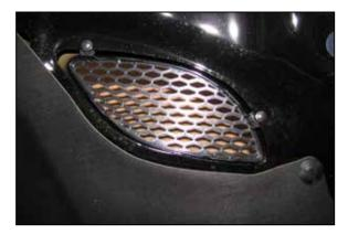
25. Some Dodge Durango models may be equipped with heat extractor vents in the hood. During inclement weather or driving in wet conditions, K&N<sup>®</sup> recommends installing the provided heat extractor block off plate. Remove the two screws that secure the factory grid in position. **NOTE: Some model may not have the screws holding in the grill.**
