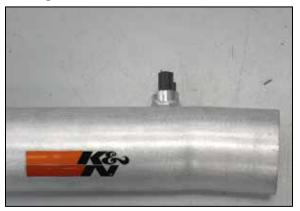
19. Install the inlet air temperature sensor into the  $K\&N^{\circledast}$  intake tube.
