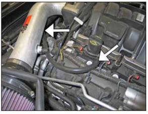
22. Install the crank case vent hose onto the 90° vent fitting and then attach the open end to the valve cover port.
