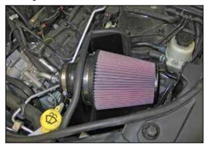
16. Install the K&N<sup>®</sup> air filter onto the adapter and secure with the provided hose clamp. NOTE: Drycharger<sup>®</sup> air filter wrap; part # RF-1041DK is available to purchase separately. To learn more about Drycharger<sup>®</sup> filter wraps or look up color availability please visit http://www.knfilters.com<sup>®</sup>.
