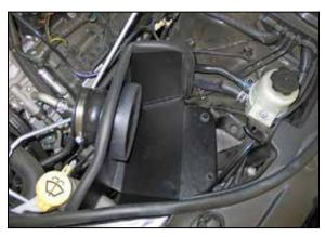
15. Set the heat shield into the vehicle so that the mounting grommets slide over the factory air box mounting studs.
