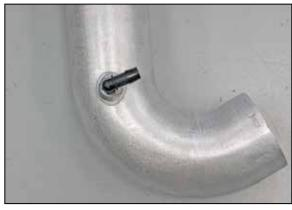
20. Install the 90° npt fitting into the K&N $^{\mbox{\tiny B}}$  intake tube as shown.
