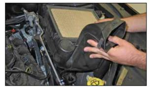
9. Lift up the lower air box to dislodge it from the mounting grommets and then remove the lower air box from the vehicle. Some vehicles may have a power steering line attached to the airbox that will need to be unhooked.
