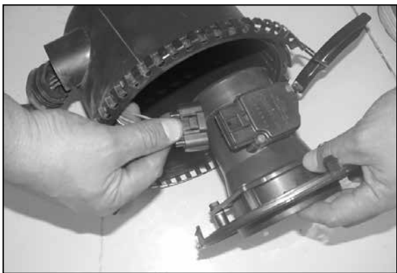
10. Pull the mass air sensor out of the housing and disconnect the mass air sensor electrical connection as shown.
