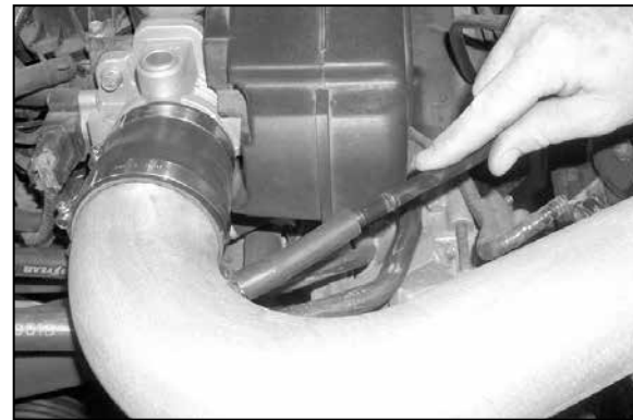
22. Reconnect the crank case vent hard line to the silicone hose on the K&N® intake tube as shown. Trim to fit if necessary.
