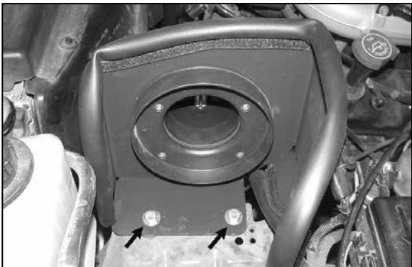
14. Secure the heat shield assembly to the stock air cleaner mounting grommets using the provided hardware as shown.
