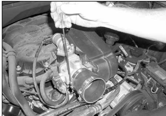
16. Install the silicone hose and hose clamps onto the throttle body and tighten as shown.
