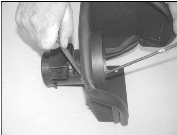
13. Assemble the provided mass air adapter, gaskets, heat shield and the stock mass air sensor using the provided hardware as shown.
