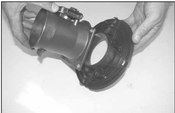
11. Remove the mass air sensor from the housing cover which is secured by two bolts.
