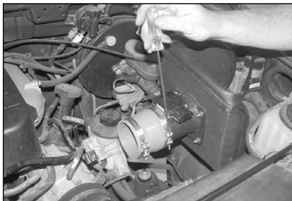
15. Install the silicone step hose and hose clamps onto the mass air sensor and tighten as shown.
