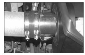
22. Install the mass air sensor assembly onto the K&N<sup>®</sup> intake tube and secure with the provided hose clamp.
