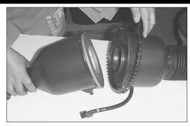
11. Open the air cleaner assembly and isolate the mass air sensor assembly.
