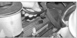
2. Rotate the crank case vent hose locking ring and pull the crank case vent hose off of the valve cover.
