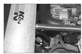
21. Install the provided silicone vent hose onto the valve cover and onto the K&N® intake tube as shown.
