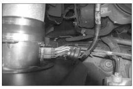
23. Reconnect the primary and secondary mass air sensor electrical connections.
