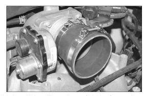
16. Install the silicone hose (084055) onto the throttle body with the hose clamps provided as
