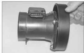
15. Attach the mass air adapter to the mass air shown.
