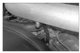
20. Attach the K&N® intake tube to the mounting bracket installed in step #17.
