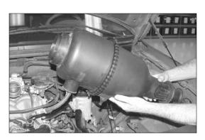
5. Pull firmly up on the air filter assembly to remove it from the mounting grommets.
