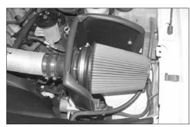
24. Install the K&N® air filter and secure with the provided hose clamp.
