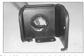
8. Install the edge trim into the hole in the heat shield as shown.
