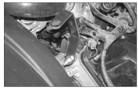
17. Install the tube mounting bracket (07198) onto the 8mm stud protruding from the engine with two flat washers and 8mm nut provided.
