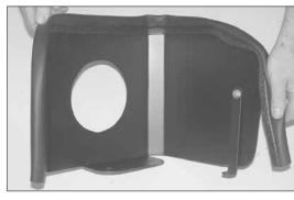
7. Install the edge trim onto the heatshield as shown. Trim if needed.
