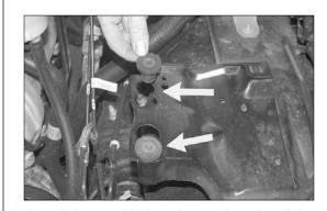
9. Install the provided nut inserts into the air box mounting holes as shown.
