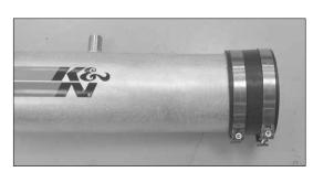
18. Install the silicone hose (08698) onto the K&N® intake tube and secure with the provided hose clamp as shown.
