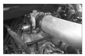
19. Install the K&N<sup>®</sup> intake tube into the silicone hose at the throttle body and secure with the provided hose clamp.
