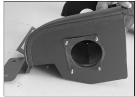
20. Install the remaining mass air sensor gasket onto the studs of the filter adapter protruding through the heat shield.
