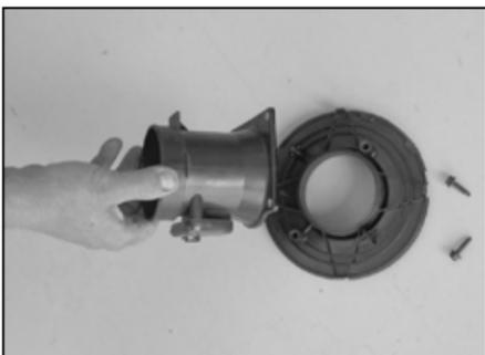
12. On 2005 and earlier vehicles, remove the two bolts that secure the mass air sensor to the mounting plate and then remove the sensor as shown.
