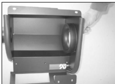
19. Install the filter adapter into the heat shield as shown.
