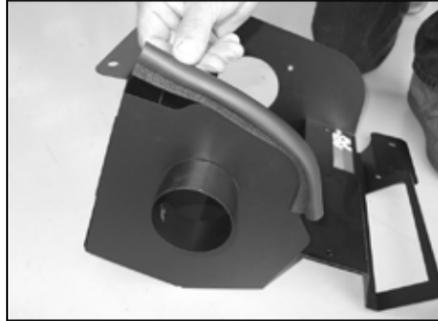
15. Install the short edge trim to the heat shield as shown. Some trimming of the edge trim may be necessary.
