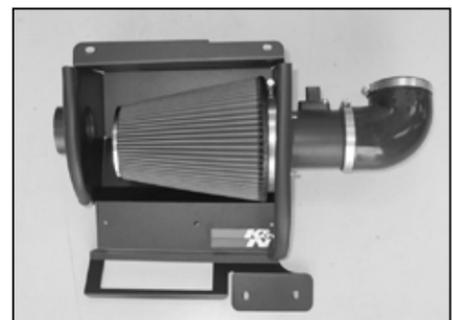
24. Install the K&N<sup>®</sup> air filter onto the filter adapter and secure with the provided hose clamp.
