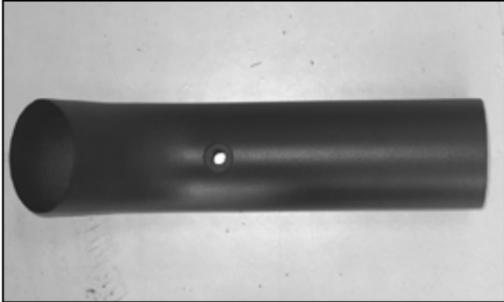
25b. Install the provided grommet into the hole drilled into the intake tube (during the previous step) as shown. Then, install the air temperature sensor into the grommet.
