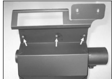
22. Install the three supplied rubber bumpers into the three holes in the heat shield from the bottom up.
