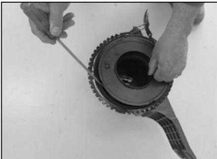
11. Use a screw driver to open the mass air sensor housing and remove the mass air sensor from the housing.
