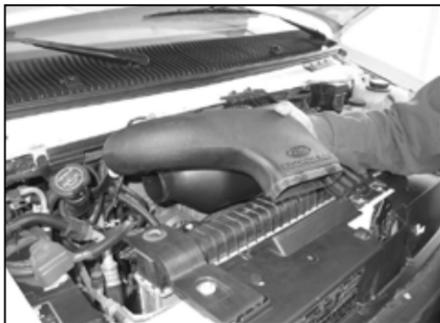
2. Unhook the fresh air intake scoop from the radiator core support and then rotate it back to unlock from the air filter assembly. Then remove it from the vehicle.
