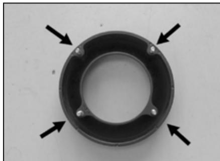
17. Install the four supplied m6 studs into the filter adapter as shown.
