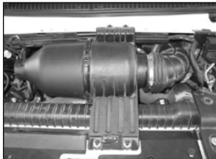
5. Remove the two bolts that secure the air filter housing to the radiator core support.
