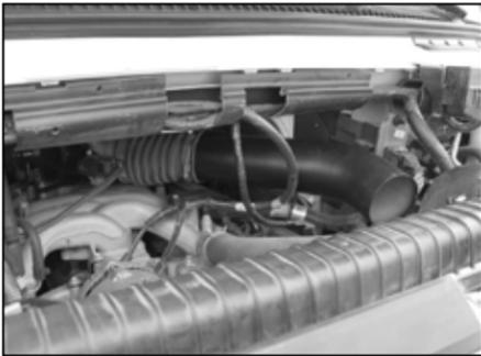
26. Install the K&N® intake tube into the bellows at the throttle body and secure with the factory hose clamp.
