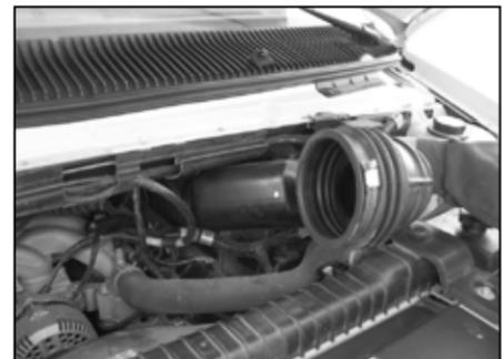
8. Remove the intake tube from the vehicle.
