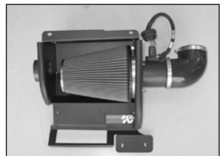
25. Reconnect the mass air sensor primary connector as shown.
