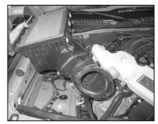
10. Lift up the lower airbox housing to dislodge it from the mounting grommets and then remove the lower airbox housing from the vehicle. **NOTE: K&N Engineering, Inc., recommends that customers do not discard factory air intake.**
