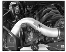
25. Install the K&N<sup>®</sup> intake tube into the silicone hose at the throttle body and align with the mounting bracket installed in step #22. Secure the intake tube with the hose clamp and supplied hardware.
