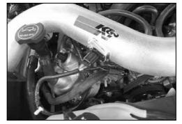
31. Reconnect the mass air sensor electrical connection.
