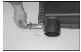
23. Remove the two screws that secure the mass air sensor to the stock airbox and then remove the mass air sensor.
