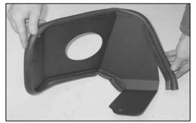
17. Install the supplied edge trim onto the heat shield as shown.
