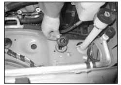
12. Remove the front lower airbox mounting grommet shown.
