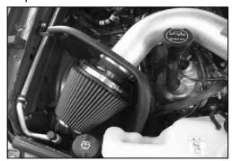
30. Install the air filter assembly onto the K&N<sup>®</sup> intake tube and secure with the provided hose clamp.
