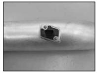
24. Install the mass air sensor assembly into the K&N $^{\odot}$  intake tube and secure with the provided hardware.
