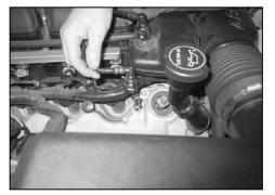
3. Disconnect the crankcase vent hose from the valve cover as shown.
