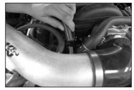
27. Install the supplied brake booster vent hose onto the factory fitting and then connect the other end to the fitting on the  $K\&N^{\otimes}$  intake tube as shown.
