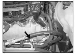
14. Remove the valve cover mounting bolt shown.
