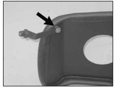
19. Attach the mounting bracket assembly to the heat shield with the provided hardware as shown. NOTE: Be sure to position the spacer between the bracket and heat shield.
