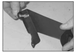
15. Insert the bolt removed in step #14 through the keyhole in the tube mounting bracket as shown.
