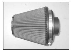
28. Install the air filter adapter into the K&N<sup>®</sup> air filter as shown and secure with the provided hose clamp.
