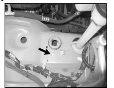
13. Remove the washer bottle mounting bolt shown.
