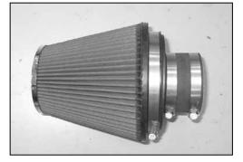
29. Install the silicone hose (08698) onto the air filter adapter and secure with the provided hose clamp.
