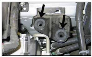
11. Remove the airbox mounting grommets shown, from the airbox mounting bracket.
