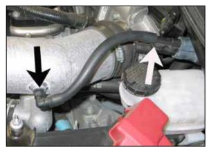
26. Attach the provided EVAP hose onto the fitting on the intake tube and then attach the open end to the EVAP check valve as shown.
