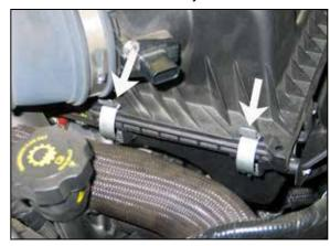
6. Release the two upper airbox latches shown.
