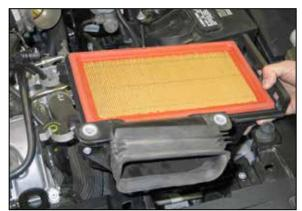
10. Lift up the lower airbox to dislodge it from the mounting grommets, then remove the lower airbox and fresh air duct from the vehicle.
