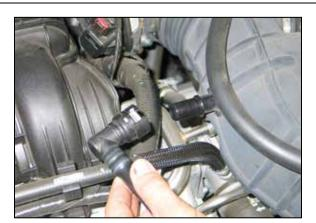
3. Release the locking tab and then disconnect crankcase vent tube from the factory intake hose as shown
