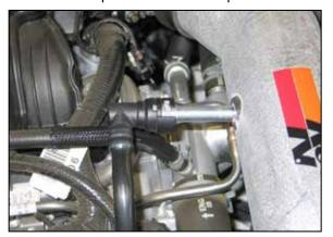
25. Connect the factory crankcase vent tube to the intake tube as shown.
