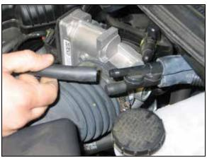
4. Disconnect the EVAP hose from the check valve as shown.
