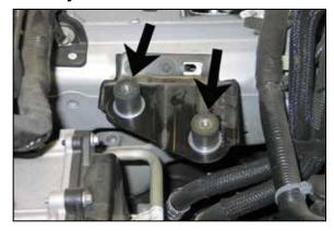
14.Install the provided rubber mounted studs onto the airbox mounting bracket as shown.
