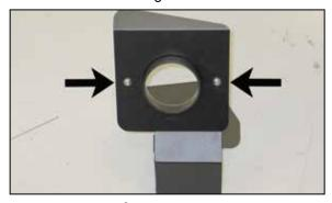
12. Install the K&N<sup>®</sup> filter adapter onto the heat shield and secure with the provided hardware.
