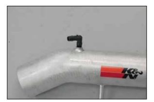
18. Install the  $90^{\circ}$  vent fitting into the intake tube as shown.
