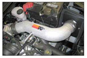
24. Install the intake tube into the silicone hose at the throttle body and onto the filter adapter, then secure with the provided hose clamps.
