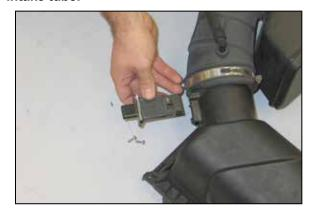
20. Remove the two screws that secure the mass air sensor to the factory airbox and then remove the sensor from the airbox as shown.
