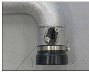
21. Install the mass air sensor into the intake tube and secure with the provided hardware.
