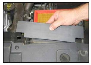
8. Remove the fresh air duct cover from the core support as shown.
