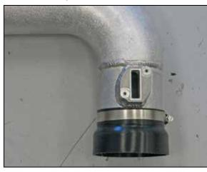
19. Install the remaining silicone hose (084073) onto the intake tube and secure with the provided hose clamp as shown.
