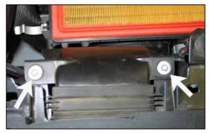
9. Remove the two bolts that secure the fresh air duct to the core support.
