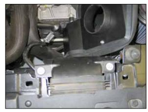
23. Install the fresh air duct into the heat shield and secure it with the factory screws in the original location, then reinstall the cover onto the core support.
