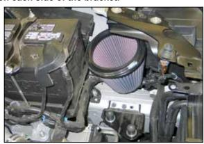
15. Set the  $K\&N^{\circledR}$  air filter into the engine compartment as shown.
