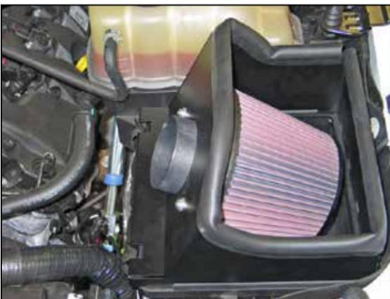
13. Install the heat shield/filter assembly onto the lower airbox and secure with the factory airbox retaining clips.
