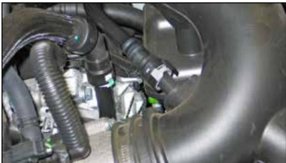
3. Rotate the locking tab and then unhook the crankcase vent hose from the factory intake tube.
