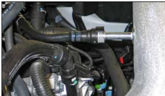
20. Connect the crankcase vent hose to the quick disconnect fitting on the K&N® intake tube.
