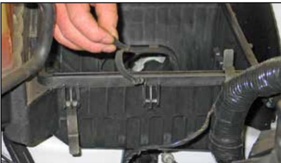
12. Remove the center airbox retaining clip.
