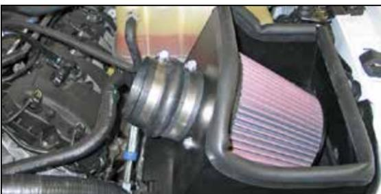
15. Install the provided silicone hose (5-576) onto the filter adapter and secure with the provided hose clamp.
