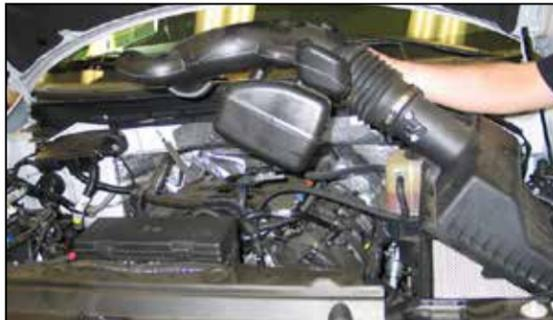
6. Release the three clips securing the upper air box housing to the lower housing and then remove the intake tube/upper airbox and air filter from the vehicle.
