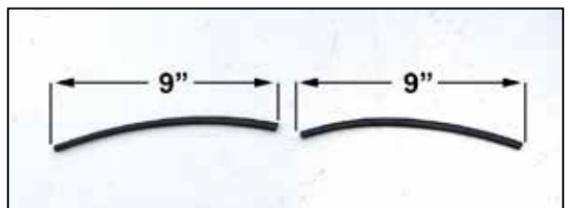
9. Cut the provided edge trim into two 9" sections as shown.
