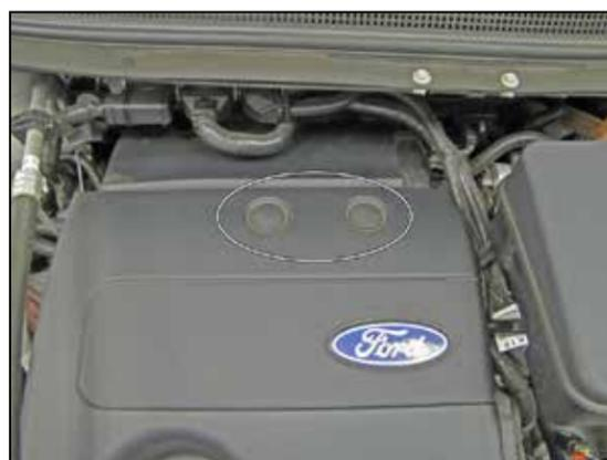
4. Remove the two push pins securing the rear of the engine cover and then remove the engine cover from the vehicle.
