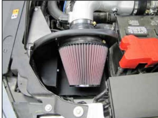
27. Install the K&N® air filter and secure with the provided hose clamp.
