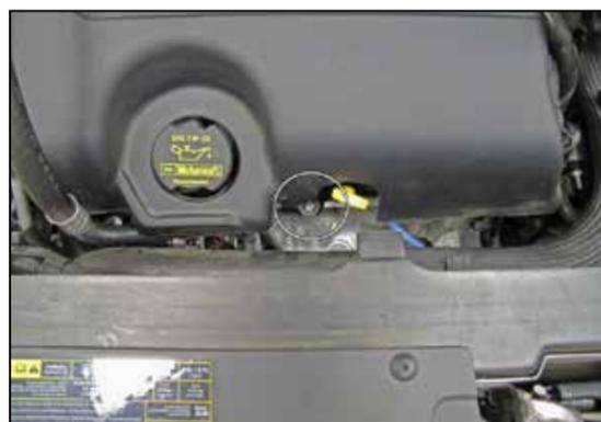
3. Remove the nut securing the front of the engine cover.
