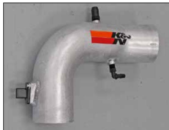
17. Install the mass air sensor into the K&N® intake tube and secure with the provide hardware.
