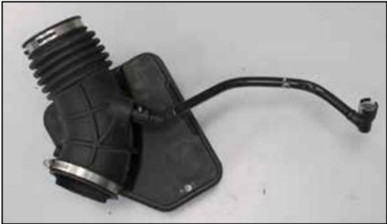
22. Rotate the locking tab and then remove the crank case vent line from the factory intake tube assembly.
