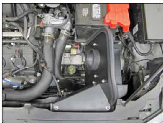
14. Install the heat shield assembly into the engine compartment so the heat shield stand-offs insert into the air box mounting grommets. Secure the fresh air intake scoop to the factory location using the provided hardware.
