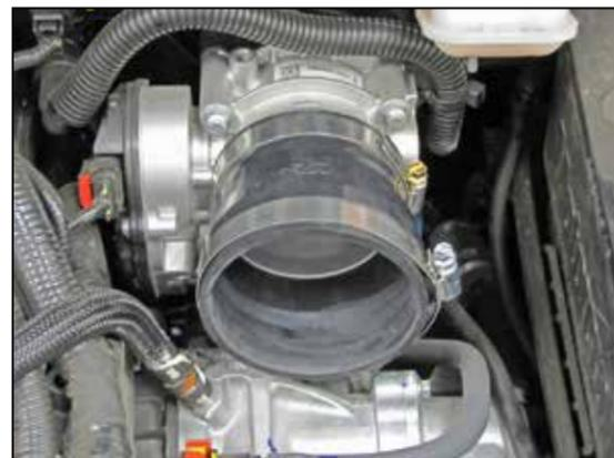
18. Install the silicone hose (08724) onto the throttle body and secure with the provided hose clamp.
