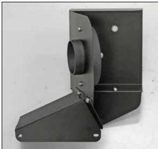
12. Install the fresh air intake scoop onto the heat shield and secure with the provided hardware.
