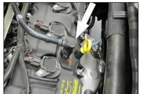
5. Rotate the locking tab and then disconnect the crank case vent tube from the valve cover.
