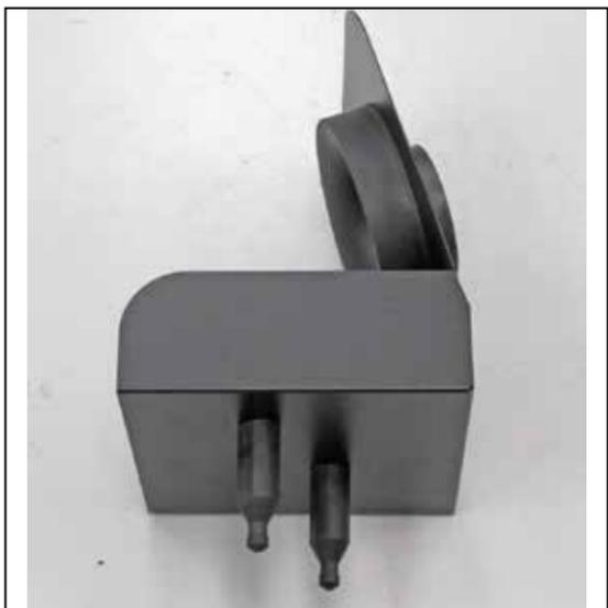
11. Install the heat shield stand-offs onto the heat shield using the provided hardware.
