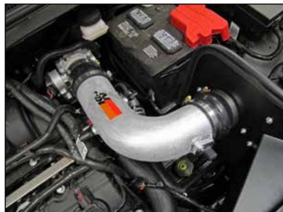
20. Install the K&N® intake tube into the silicone hose at the throttle body then align with the filter adapter, slide the silicone hump hose onto the filter adapter. Secure the intake tube with the provided hose clamps.
