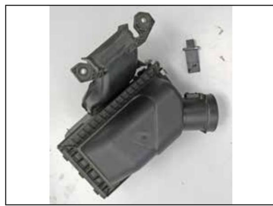
16. Remove the two screws securing the mass air sensor into the factory air box and then remove the mass air sensor from the air box.
