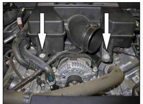
6. Remove the two bolts securing the intake plenum onto the intake manifold.
