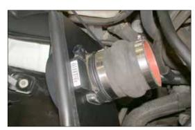
15. Install the silicone step hump hose and hose clamps onto the mass air sensor and tighten as shown.
