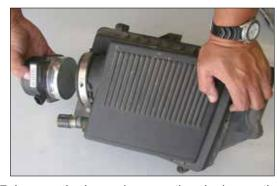
7. Loosen the hose clamp on the air cleaner then remove the mass air sensor as shown.
