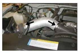
16. Install the K&N® Intake tube into the angled hose, then, slide the other end into the hump hose. Adjust everything for best fit and clearance then tighten the hose clamps as shown.
