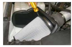
18. Install the K&N® air filter onto the mass air adapter and secure with the provided hose clamp as shown.
