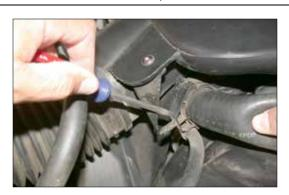
4. Unclip the radiator hose from the intake tube as shown.
