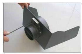
10. Using the provided hardware assemble the mass air adapter, heat shield, gaskets, and the stock mass air sensor as shown.
