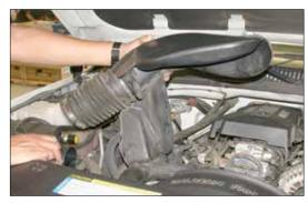
5. Disconnect the stock intake tube from the mass air sensor and from the throttle body, then, remove the intake tube as shown.
