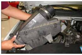
6. Pull firmly upwards to remove the air cleaner assembly as shown.
