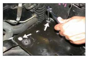
8. Remove the two stock air cleaner support tray bolts as shown.
