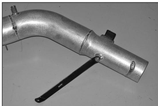
17. Install the small end of the tube-mounting bracket on the K&N® intake tube as shown.
