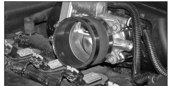
9. Install the silicone hose (08051) onto the throttle body and secure with the provided hose clamps as shown.
