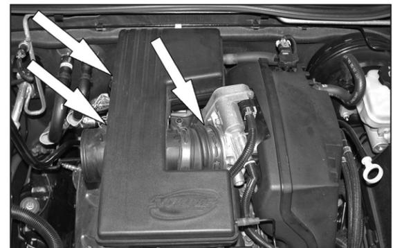
7. Loosen the two bolts that retain the intake resonator to the engine, and then loosen the hose clamp at the throttle body.
