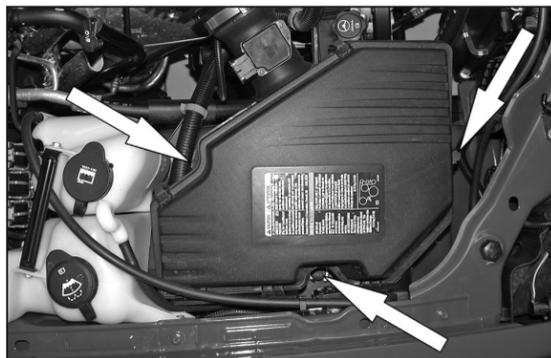
4. Loosen the two air box retaining bolts and one retaining nut.
