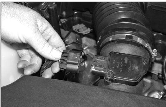
2. Depress the locking clip on the mass air sensor electrical connection, and then separate the mass air sensor electrical connection.
