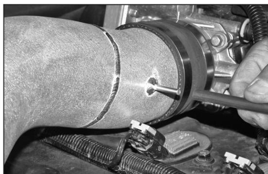
20. Install the provided 4mm vacuum hose onto the fuel pressure regulator, then onto the vent fitting on the K&N® intake tube.
