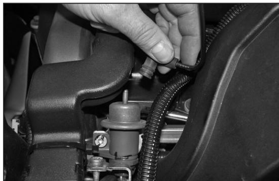
6. On vehicles equipped with a fuel pressure regulator disconnect the fuel pressure regulator vacuum hose from the fuel pressure regulator as shown.
