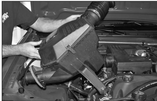
5. Lift up the air box and remove it from the vehicle.
