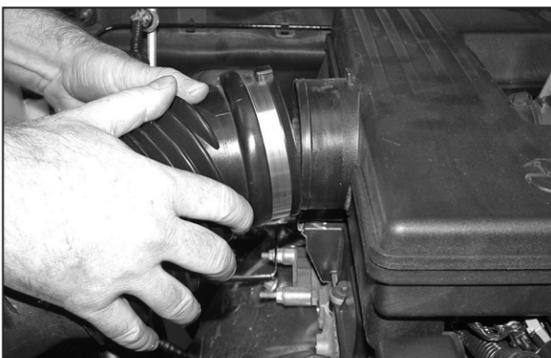
3. Loosen the hose clamp that retains the stock intake tube to the resonator, and then remove the tube from the resonator as shown.
