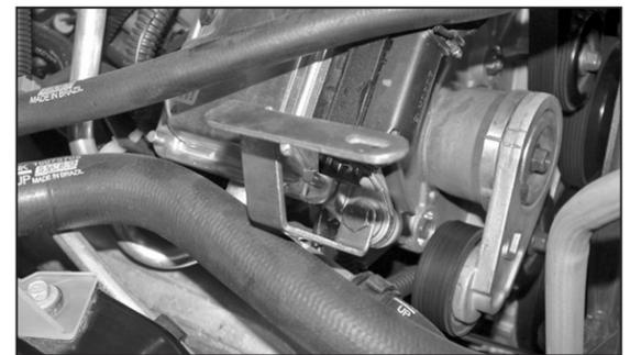
7. Using the factory bolt removed in step #6, install the tube mounting bracket to the engine processor as shown.
