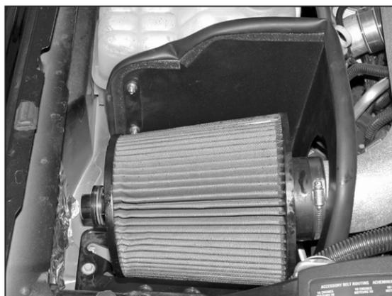
19. Install the K&N® Air filter onto intake tube as shown then tighten completely.
