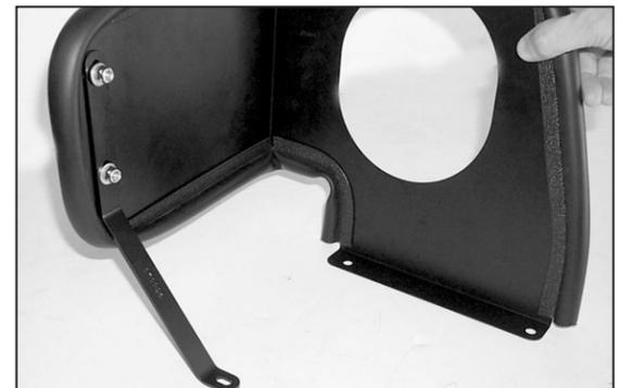
9. Install bracket onto heat shield as shown. Do not tighten completely.
