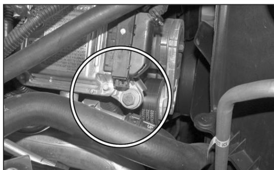
6. Remove the lower front engine processor mounting bolt shown.
