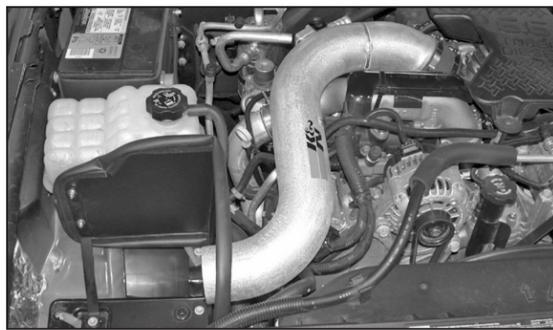
15. Install the K&N® intake tube into the silicone hose at the intake inlet, then align the tube to the mounting bracket installed in step #7 and secure with the provided hardware.
