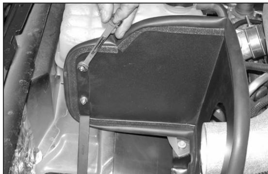
16. Adjust heat shield and bracket for necessary clearance, then tighten all hardware completely.
