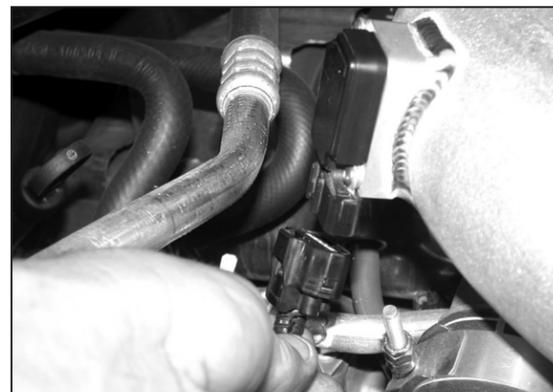
20. Reconnect the mass air sensor electrical connection as shown.
