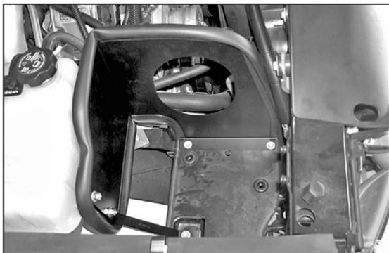
11. Mount the heat shield onto the airbox mounting tray and secure with the three bolts removed in step 10.
