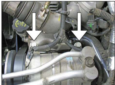
17. Remove the two A/C compressor pump mounting bolts mounting bolts shown.
