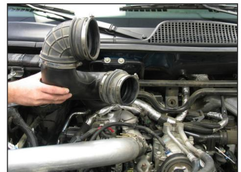
7. Loosen the hose clamp that secures the stock intake tube to the turbo inlet tube. Then remove the complete intake tube assembly from the vehicle as shown.
