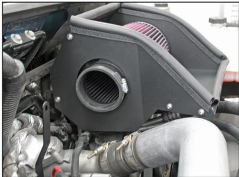
26. Install the heat shield side panel onto the main heat shield and secure with the provided hardware.
