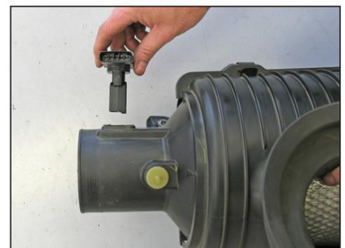
8. Remove the two screws that secure the mass air sensor to the stock filter housing and then remove the mass air sensor as shown.
