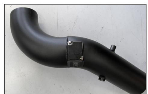
9. Install the mass air sensor into the secondary K&N® intake tube and secure with the provided hardware.
