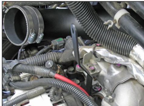
16. Install the secondary tube mounting bracket (26650) onto the intercooler manifold mounting stud and secure with the nut removed in step #15.
