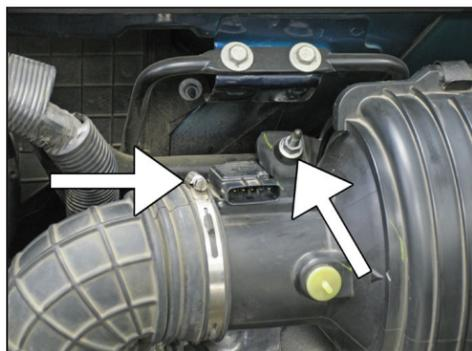
4. Loosen the hose clamp that secures the stock intake tube to the filter housing and then remove the nut that secures the filter housing to the support bracket.
