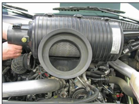
6. Remove the filter housing from the vehicle.
