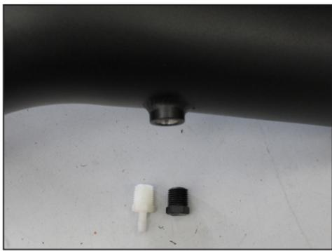
10. On vehicles equipped with a filter minder, install the 1/4" npt vacuum fitting into the K&N® intake tube. On vehicles without a filter minder, install the 1/4" npt plug into the K&N® intake tube.
