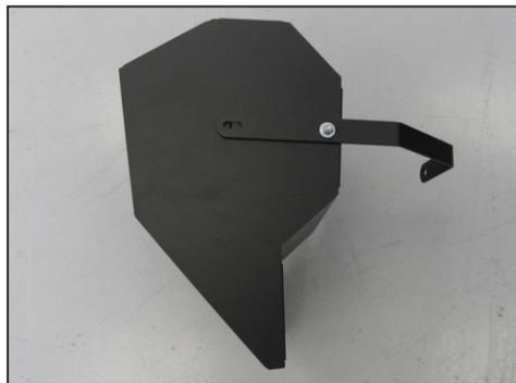
19. Install the heat shield mounting bracket onto the heat shield and secure with the provided hardware as shown.
