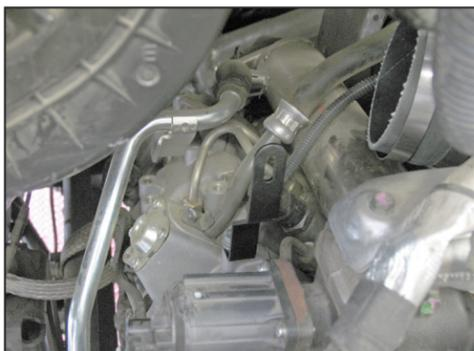
12. Install the primary tube mounting bracket (26645) onto the engine valve cover as shown with the provided hardware.
