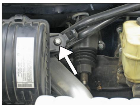
5. Remove the bolt that secures the filter housing to the support brace shown.
