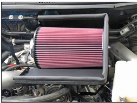
25. Install the K&N® air filter into the heat shield so the mounting stud protrudes through the heat shield and the mounting bracket. Then secure the filter with the supplied hardware.
