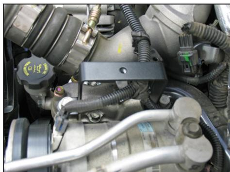
18. Install the heat shield mounting bracket (26644) onto the A/C compressor and secure with the bolts removed in step #17.
