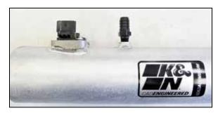
16. Install the mass air sensor into the K&N intake tube and secure with the provided hardware. Install the provided CCV fitting into the K&N intake tube as shown. NOTE: NPT fittings have tapered threads, hand tighten then rotate 1 revolution with a wrench until tight and difficult to turn. Over tightening will damage the fitting and tube.
