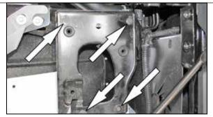
7. Remove the four bolts securing the air box mounting tray and then remove the tray from the vehicle. NOTE: Three of the bolts will be reused in a latter step.
