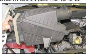
6. Pull up the air box to release it from the mounting grommets and then remove the factory air box from the vehicle.
