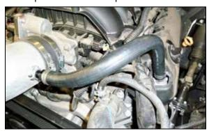
19. Install the provided CCV hoses onto the valve cover ports and connect the driver side hose to the K&N intake tube and secure with the provided hose clamps.
