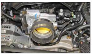
13. Install the coupling hose (08698 for 5.3L, 08497 for 6.2L) onto the throttle body and secure with the provided hose clamp.
