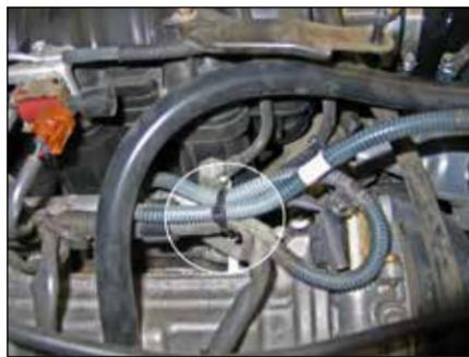
30. Using the provided wire tie, secure the excess mass air wire to the tube-mounting bracket as shown.
