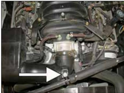
4. Loosen and remove the bolt that secures the A/C hose to the stock intake tube. **NOTE: This bolt will be reused in a later step.**
