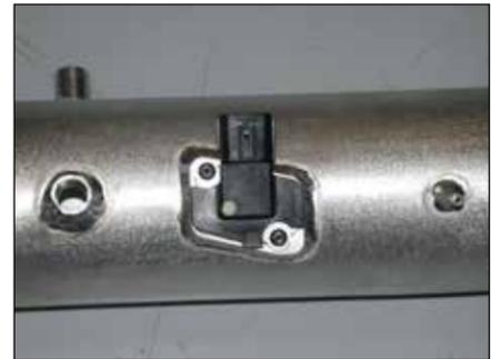
10. Install the mass air sensor into the K&N® intake tube and secure with the provided hardware as shown.
