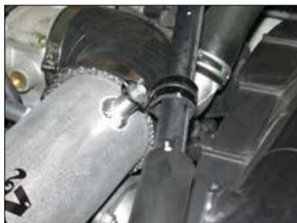
20. Attach the A/C hose to the intake tube with the bolt removed in step #4.
