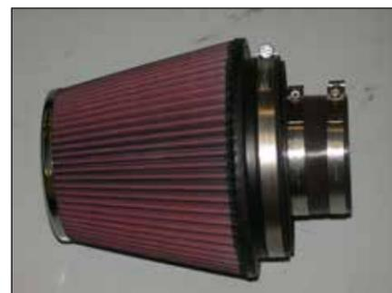
26. Install the silicone hose (08698) onto the filter adapter as shown and secure with the provided hose clamp.
