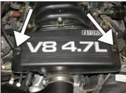
3. Loosen and remove the nuts shown that secure the throttle body cover, then remove the throttle body cover from the engine. **NOTE: The mounting nuts will be reused.**
