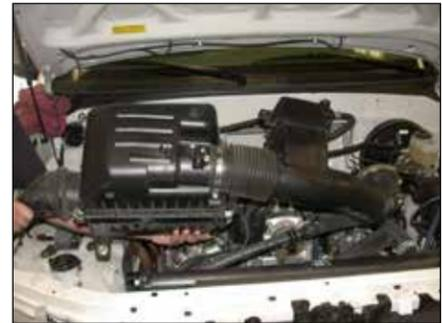
8. Remove the complete intake assembly from the vehicle as shown. **NOTE: K&N Engineering, Inc., recommends that customers do not discard factory air intake.**
