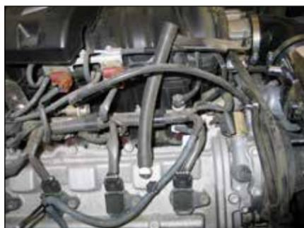
21. Remove the factory crankcase vent hose and fuel pressure regulator vent hose shown from the engine.
