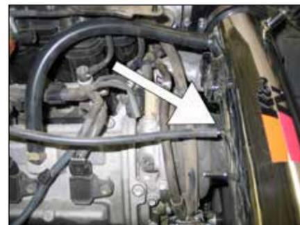
23. Install the provided fuel pressure regulator vent hose onto the fuel pressure regulator and then attach to the K&N® intake tube as shown.
