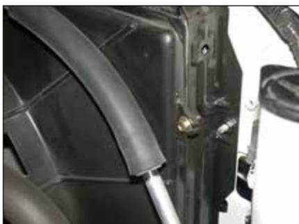
15. Remove the radiator fan shroud upper mounting bolt shown.
