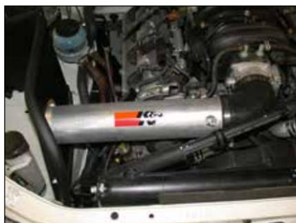
19. Install the intake tube onto the throttle body and align the tube mounting bracket with the threaded boss on the engine, then secure with the provided hardware.
