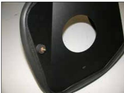
12. Install the rubber mounted stud onto the heat shield as shown using the provided hardware.
