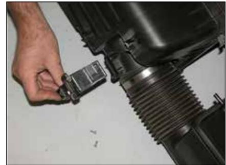
9. Remove the two screws which secure the mass air sensor to the factory air box, then remove the mass air sensor from the air box as shown.
