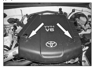
32. Install the engine cover and secure with the factory mounting nuts removed in step #2.
