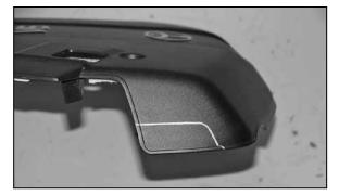
31. Using the provided template, mark the trim lines onto the engine cover and then cut with the appropriate tool.
