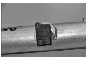
19. Install the mass air sensor into the K&N® intake tube with the hardware provided.
