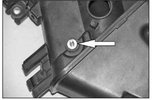
29. Using a pair of pliers, remove the engine covermounting stud shown from the factory air box.
