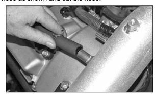
24. Reinstall the crank case vent hose into the valve cover and then connect the cut end to the  $K\&N^{@}$  intake tube as shown. Secure the vent hose with the factory spring clamps.
