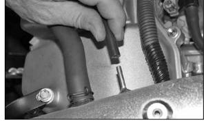
25. Remove the stock vacuum hose from the fuel pressure regulator, then install the provided silicone hose to the fuel pressure regulator and then onto the K&N® intake tube as shown.
