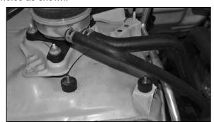
14. Install the two remaining rubber mounted studs to the original air box mounting holes as shown.
