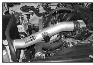
21. Install the K&N® intake tube into the silicone hose at the throttle body and align the mounting stand off with the bracket installed in step #20. Secure the intake tube with the hose clamp and hardware provided.
