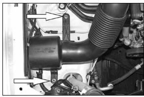
4. Remove the two bolts which secure the intake resonator to the fender well.
