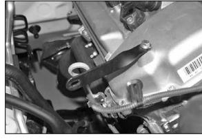
20. Install the tube mounting bracket onto the threaded boss on the valve cover with the provided hardware as shown.
