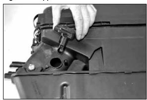
18. Remove the two screws that secure the mass air sensor to the air box assembly, then remove the mass air sensor as shown.
