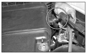
8. Remove fuel pressure regulator hose from back side of air box.
