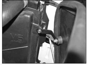
16. Secure the mounting bracket to the fan shroud with the original bolt.
