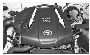
2. Loosen the two nuts that secure the engine cover, and then remove the engine cover from the engine.
