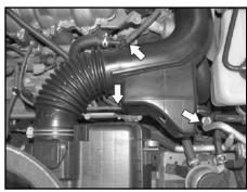
4. Remove the three vent lines from the air intake resonator as shown.
