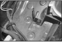
8. Remove the 12mm bolt that retains the power steering reserve to vehicle then mount the provided bracket (07158) onto the vehicle with the bolt that was removed.
