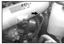
19. Connect the factory power steering pressure switch vent hose onto the K&N<sup>®</sup> intake tube as shown.
