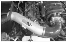
16. Install the K&N<sup>®</sup> intake tube into the throttle body and align with the mounting bracket installed in step #12. Secure with the provided hardware.
