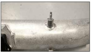
20. Install the engine cover mounting stud into the K&N<sup>®</sup> intake tube as shown.
