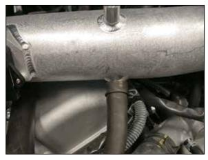
27. Connect the crank case vent hose to the K&N<sup>®</sup> intake tube and secure with the stock hose clamp.
