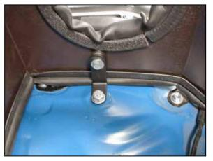
16. Secure the bottom of the heat shield to the inner fender with the small "L" bracket. NOTE: Be sure to us the provided spacer between the bracket and heat shield.
