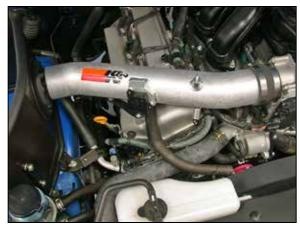
23. Install the intake tube into the silicone hose at the throttle body and align the mounting bracket with the threaded boss on the valve cover, then secure with the provided hardware and hose clamp.
