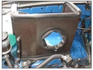
14. Install the heat shield into the vehicle and secure to the power steering reservoir with the bolt removed in step #13.
