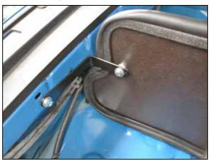
15. Secure the heat shield to the inner fender with the large "L" bracket as shown.
