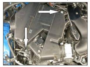
8. Remove the two air box mounting bolts shown and loosen the hose clamp at the throttle body.
