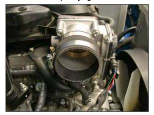
22. Install the supplied silicone hose (08434) onto the throttle body and secure with the provided hose clamp.
