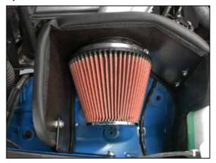
26. Install the K&N<sup>®</sup> filter assembly onto the K&N<sup>®</sup> intake tube and secure with the provided hose clamp.
