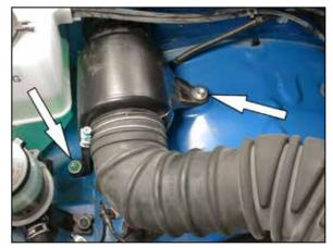
6. Remove the two intake resonator mounting bolts shown.
