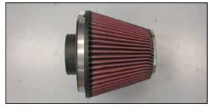
24. Install the provided filter adapter into the K&N<sup>®</sup> filter as shown and secure with the provided hose clamp.
