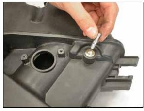
19. Remove the engine cover mounting stud from the factory air box.
