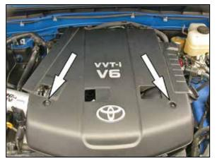
30. Reinstall the engine cover and secure with the factory mounting nuts.
