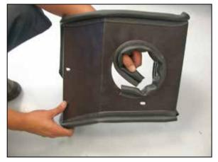
11. Install the short edge trim to the inside of the intake tube pass trough hole as shown. NOTE: some trimming of the edge trim may be necessary.
