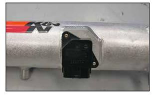
18. Install the mass air sensor into the K&N® intake tube using the provided hardware.
