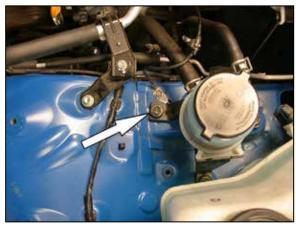
13. Remove the power steering reservoir mounting bolt shown.
