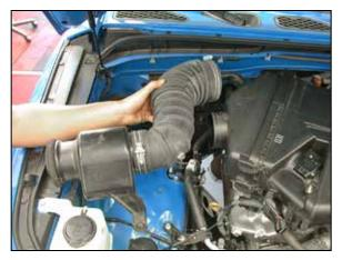
7. Loosen the hose clamp which secures the intake tube to the stock air filter housing and then remove the intake tube and resonator assembly.
