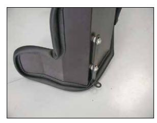
12. Install the mounting bracket (07159) onto the heat shield using the provided spacers as shown.
