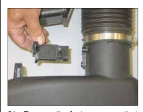
21. Remove the factory screws that secure the mass air sensor to the factory intake tube, and then remove the mass air sensor from the stock intake tube.
