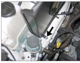
18. Secure the front heat shield bracket to the front air box mounting location with the provided hardware.
