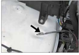
16. Remove the bolt that retains the ground strap to the inner fender.
