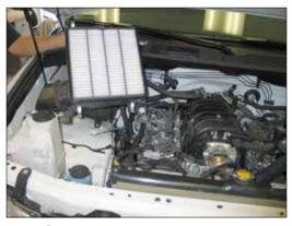
8. Lift the lower air box up, releasing it from the inner fender mounting grommet and fresh air duct. Remove the lower air box from the vehicle.
