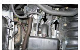
5. Disconnect the fuel pressure regulator hose from the fuel pressure regulator. Disconnect the crank case vent hose from the valve cover.
