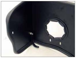
13. Install the provided "C" (#07190) bracket onto the heat shield with the provided hardware as shown.
