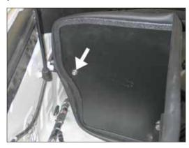
19. Secure the rear of the heat shield to the bracket installed in step #11.
