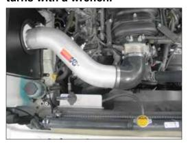
24. Install the K&N<sup>®</sup> intake tube into the silicone hose at the throttle body and align with the mounting bracket installed during step #10. Secure the intake tube with the hose clamp and hardware provided.
