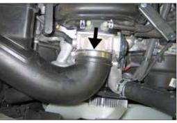
4. Loosen the hose clamp that secures the stock intake tube to the throttle body.
