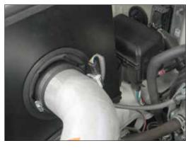
28. Reconnect the mass air sensor electrical connection as shown.
