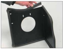
10. Install the long edge trim onto the heat shield as shown.
