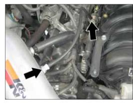
26. Install the provided fuel pressure hose onto the fuel pressure regulator and then connect the open end onto the remaining NPT fitting installed into the K&N® intake tube as shown.
