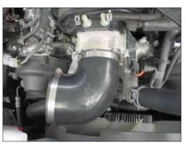
20. Install the silicone hose (#084086) onto the throttle body and secure with the provided hose clamp.
