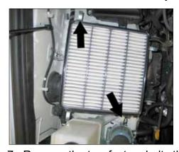
7. Remove the two factory bolts that secure the lower air box to the inner fender.
