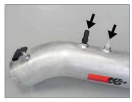
23. Install the provided ½"npt fittings into the K&N® intake tube as shown.
