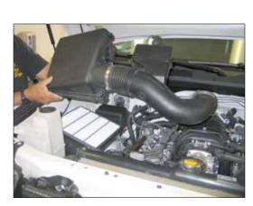
6. Release the four upper air box clam shell clamps, then remove the upper airbox and intake tube assembly.
