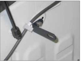
9. Install the small "L" bracket (#070742) onto the inner fender, behind the hood support. Secure with the provided hardware as shown.
