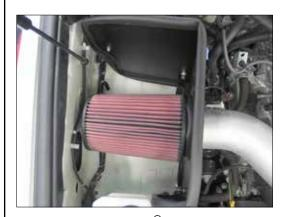
27. Install the K&N<sup>®</sup> air filter onto the K&N<sup>®</sup> intake tube and secure with the provided hose clamp.
