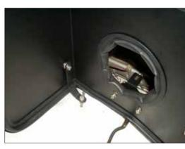
17. Set the heat shield into position on the inner fender. Secure the "C" bracket to the ground strap location.
