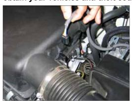
2. Disconnect the mass air sensor electrical connection. Then unclip the mass air sensor wiring harness from the air box.
