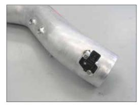
22. Install the mass air sensor into the K&N<sup>®</sup> intake tube and secure with the provided hardware.
