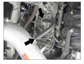
25. Install the provided crank case vent hose onto the valve cover fitting, and then connect the open end to the NPT fitting installed into the K&N® intake tube as shown.
