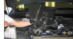
2. Remove the two nuts shown that secure the engine cover and then remove the engine cover.
