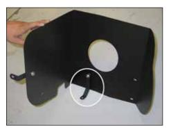
10. Install the "L" bracket (07190) onto the heat shield as shown using the provided hardware. NOTE: Place the provided spacer between the bracket and heat shield.
