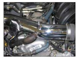
27. Install the engine cover mounting stud into the  $K\&N^{\otimes}$  intake tube as shown.
