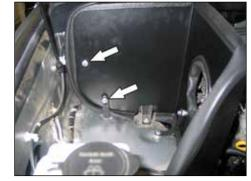
17. Secure the rear of the heat shield to the bracket installed in step #12 using the hardware and spacer provided. Secure the heat shield to the upper bracket with the hardware provided.
