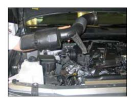
4. Remove the fresh air intake tube from the engine compartment as shown.
