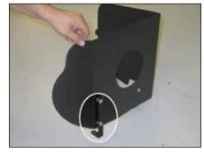
11. Install the "L" bracket (070902) onto the heat shield as shown using the provided hardware. NOTE: Place the provided spacers between the bracket and heat shield.
