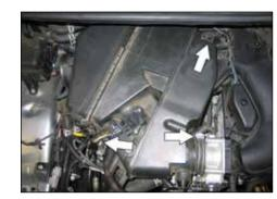
7. Loosen the hose clamp at the throttle body and then remove the two air box mounting bolts shown.
