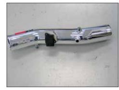
23. Install the mass air sensor into the K&N^ ${\rm \$}$  intake tube and secure with the provided bolts.
