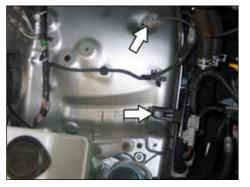
15. Remove the ground strap mounting bolt and the air injection mounting bracket nut shown. **NOTE: The nut will be reused in a later step.**
