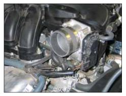
21. Install the provided silicone hose (08711) onto the throttle body and secure with the provided hardware. 26. Reconnect the crank case vent hose to the  $K\&N^{\text{(s)}}$  intake tube as shown.
