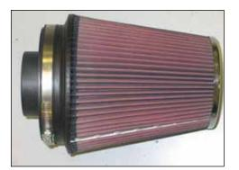
28. Install the filter adapter into the K&N<sup>®</sup> air filter and secure with the provided hose clamp.
