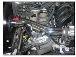
25. Install the K&N<sup>®</sup> intake tube assembly into the silicone hose at the throttle body and align with the tube mounting bracket , then secure with the provided hose clamp and hardware.
