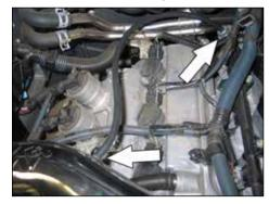
31. Install the provided vacuum hose onto the fuel pressure regulator and then attach the open end to the vent fitting on the  $K\&N^{\otimes}$  intake tube.
