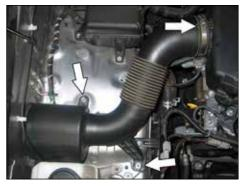
3. Loosen the fresh air intake tube hose clamp and remove the two mounting bolts.
