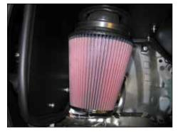
30. Install the filter assembly onto the K&N<sup>®</sup> intake tube and secure with the provided hose clamp.
