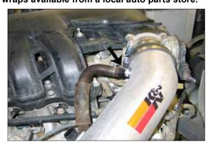
27. Connect the crank case vent line to the 5/8 vent fitting and secure with the factory spring clamp.
