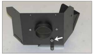
15. Install the provided mounting bracket (070712A) onto the heat shield and secure with the provided hardware.
