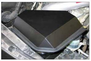
31. Install the heat shield cover onto the heat shield and secure with the provided hardware.
