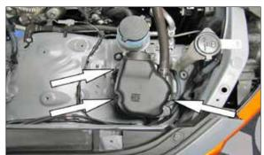
11. On models with the Air injection pump located in front of the air box next to the Power steering reservoir, remove the three bolts securing the pump to the inner fender.
