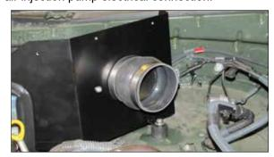
20. Install the provided silicone hump hose (084057) onto the filter adapter and secure with the provided hose clamp.
