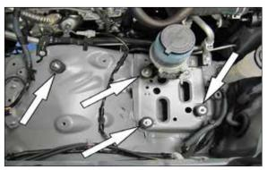
12. Install the four rubber mounted studs into the factory air box and P/S reservoir as shown.
