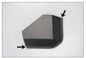
30. Install the remaining 19" piece of edge trim onto the heat shield cover as shown.
