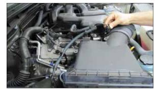
3. Disconnect the mass air sensor electrical connection and then unhook the wiring harness from the air box. **NOTE: The wiring harness attaches in three locations.**
