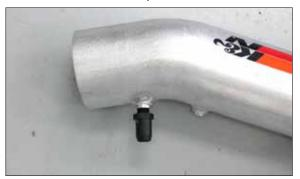
24. Install the 5/8 vent fitting into the K&N® intake tube as shown.
