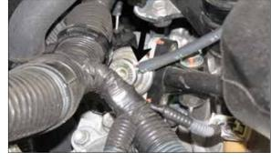
4. Unhook the fuel pressure vent line from the fuel pressure regulator.
