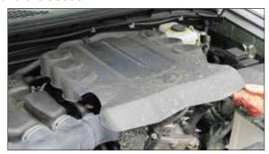
2. Lift up the engine cover to dislodge it from the mounting grommets and then remove the cover from the vehicle.
