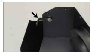
16. Install the provided mounting bracket (08022) onto the heat shield and secure with the provided hardware.
