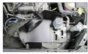
19. Set the heat shield onto the rubber mounted studs and the secure with the provided hardware. NOTE: On models that had a horn attached in this location, be sure to reattach the horn between the heat shield bracket and rubber mounted stud.
