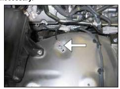
18. Remove the bolt that secures the ground strap to the inner fender.
