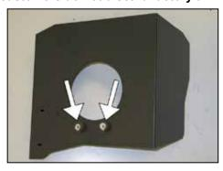
11. Install the two rubber mounted studs onto the heat shield using the provided hardware as shown.
