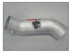
21. Install the mass air sensor into the  $K\&N^{\rm @}$  intake tube and secure with the provided hardware.
