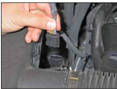
5. Disconnect the mass air sensor electrical connection and unhook the wiring harness from the upper airbox.
