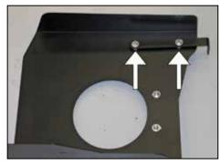
12. Install the heat shield mounting bracket (070902A) onto the heat shield using the provided hardware and spacers as shown.
