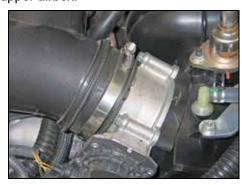
6. Loosen the hose clamp that secures the factory intake tube to the throttle body.
