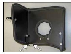
17. Install the provided longer edge trim onto the heat shield as shown.
