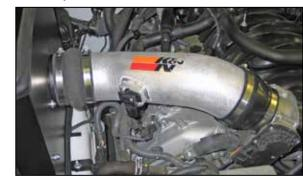
22. Install the K&N® intake tube into the hump hose attached to the heat shield and then into the step hose attached to the throttle body. Secure with the provided hose clamps.
