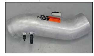
19. Install the provided NPT vent fittings into the  $K\&N^{\circledcirc}$  intake tube as shown.
