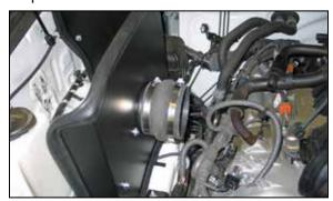
16. Install the silicone hump hose (08418) onto the filter adapter and secure with the provided hose clamp.
