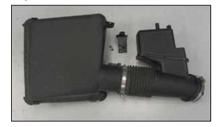
17. Remove the two screws securing the mass air sensor. Remove the mass air sensor from the upper air box housing.
