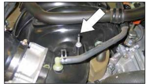
26. Remove the front engine cover mounting stud from the intake manifold.
