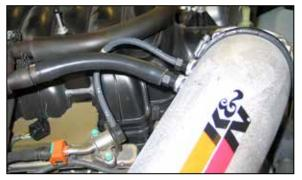
23. Connect the crank case vent hose and the fuel pressure hose to the fittings connected to the K&N® intake tube.
