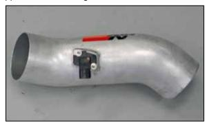
18. Install the mass air sensor into the intake tube and secure with the provided hardware.
