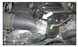
4. Loosen the hose clamp that secures the intake tube to the throttle body.
