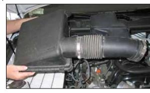
6. Release the four retaining clips securing the upper air box, then remove the upper air box and intake tube assembly from the vehicle.
