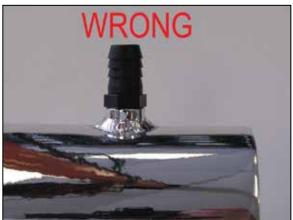
**17.** Install the provided vent fitting "hand" tight, then tighten 1-1/2 rotations into the K&N intake tube as shown. Do not bottom out fitting.
