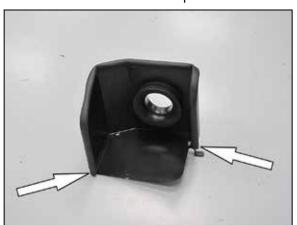
11. Install the provided edge trim onto the  $K\&N^{\otimes}$  heat shield as shown.
