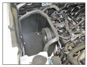
12. Install the heat shield onto the rubber mounted studs installed in the earlier step and secure with the provided hardware.
