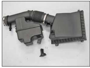
15. Remove the mass air sensor from the factory air filter housing.
