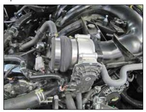
13. Install the provided hump coupler (08171) onto the throttle body and secure with the provided hose clamp.
