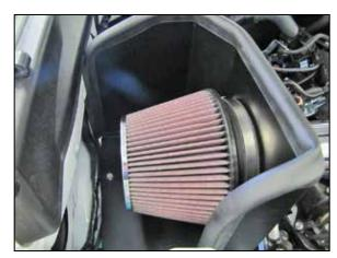
21. Install the K&N® air filter onto the filter adapter and secure with the provided hose clamp. NOTE: Drycharger® air filter wrap; part # 22-8049DK is available to purchase separately. To learn more about Drycharger® filter wraps or look up color availability please visit http://www.knfilters.com®.
