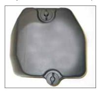
2. Loosen the air cleaner cover knobs and remove the cover.
