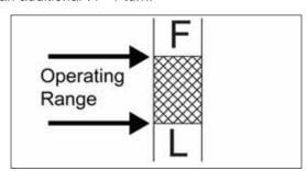
8. Fill the engine with the Lucas® 30WT Plus Engine Oil to the Full or "F" mark on the dipstick. Always check the oil level with the dipstick before adding more oil.
