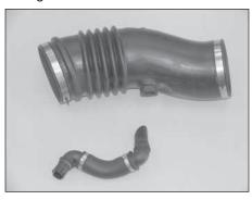
23a. On 2006 and later vehicles, cut the band clamp which secures the crank case vent tube to the turbo inlet tube. Then remove the crank case tube assembly from the turbo inlet tube as shown.
