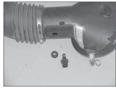
11. On vehicles equipped with an air temperature sensor, remove the air temperature sensor and grommet as shown.
