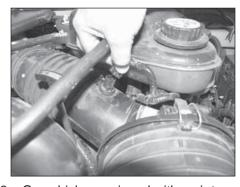
3a. On vehicles equipped with a air temperature sensor, disconnect the temperature sensor electrical connection as shown.
