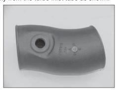
23b. On 2006 and later vehicles, install the provided grommet into the K&N® turbo inlet tube as shown.
