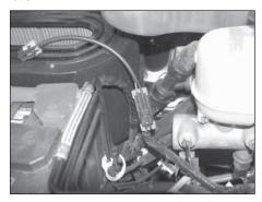
25. Install the provided wiring harness extension to the factory wiring harness filter minder connection as shown.
