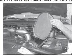
7. Remove the filter housing from vehicle as shown.
