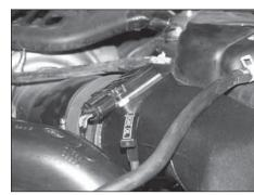
28. On vehicles equipped with a mass air sensor, connect the mass air sensor electrical connection. On vehicles equipped with an air temperature sensor, reconnect the air temperature sensor electrical connection.
