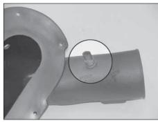
13. On vehicles equipped with the air temperature sensor, install the factory grommet and temperature sensor removed in step #11 into the K&N® intake tube at the hole drilled in step #12.
