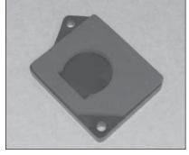
14. On vehicles equipped with an air temperature sensor, install the provided gasket onto the mass air block off plate as shown.
