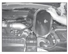
8. Remove the air box base as shown.
