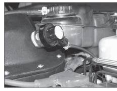
29. Connect the filter minder jumper harness into the filter minder as shown.
