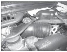
9a. On 2006 and later vehicles, loosen the hose clamp which secures the intake bellows and tube assembly to the turbo inlet.
