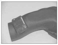
18. On vehicles equipped with the mass air sensor install the mass air sensor onto the K&N® air box lid with the provided screws and spacers as shown.
