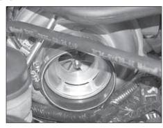
9d. On 2006 and later vehicles, install the silicone hose (08761) onto the turbo inlet and secure with the provided hose clamp.
