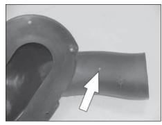
12. On vehicles equipped with an air temperature sensor, drill a 5/8" hole into the K&N® air box lid at the drill point shown.
