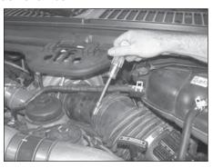
5. Loosen the hose clamp at the turbo inlet tube which secures the intake bellows as shown.
