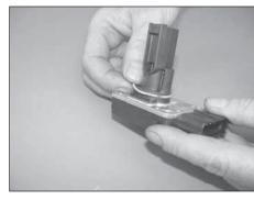
16. On vehicles equipped with a mass air sensor remove the factory O ring from the mass air sensor as shown.
