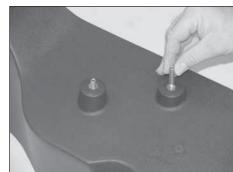
21. Install the two 8mm studs into the mounting boss on the bottom of the  $K\&N^{\otimes}$  air box base as shown.
