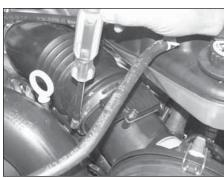
5a. On 2006 and later vehicles, loosen the hose clamp which secures the intake bellows and tube assembly to the rear air filter housing as shown.
