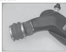
26. Install the silicone hose (08613) onto the K&N® air box lid with the provided hose clamp as shown.
