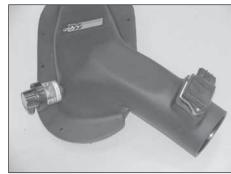
20. Install the factory grommet and restriction gauge into the  $K\&N^{\tiny{\circledR}}$  air box lid as shown.
