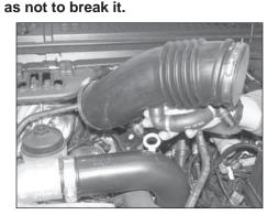
9c. On 2006 and later vehicles, remove the intake bellows and tube assembly from the vehicle as shown.
