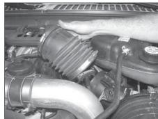
6. Loosen the hose clamp at the mass air sensor, then remove the intake hose from the vehicle.
