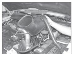
Remove the air box top as shown.
