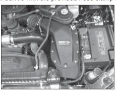
27. Install the K&N® air box lid onto the air box base making sure the silicone hose is completely installed onto the intake inlet. Install all ten air box lid mounting nuts and washers onto the lid. Once all the nuts are installed they can be tightened completely. Tighten the hose clamp, which secures the silicone hose to the throttle body.
