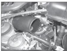
23d. On 2006 and later vehicles, install the K&N® turbo inlet tube assembly onto the turbo; rotate to align the crank case vent tube until it aligns with the vent port in the valve cover. Then snap the crank case vent tube into the valve cover and secure the tube with the provided hose clamp.
