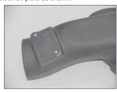
15. On vehicles equipped with an air temperature sensor, install the mass air block off plate onto the K&N® intake tube using the provided screws and spacers as shown.
