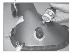
19. Remove the air filter restriction gauge and grommet from the factory air box.
