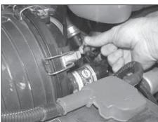
2. Disconnect the restrictor gauge electrical connection as shown.
