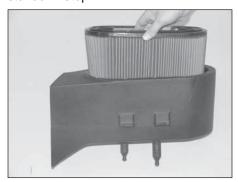
23. Install the K&N® air filter into the K&N® air box housing as shown.
