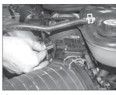
3. On vehicles equipped with a mass air sensor disconnect the mass air electrical connection as shown.
