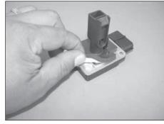
17. On vehicles equipped with a mass air sensor install the provided gasket onto the mass air sensor with the sticky side down.
