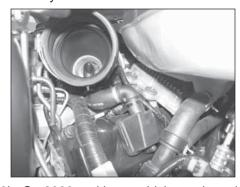
9b. On 2006 and later vehicles, using a large screwdriver, pry up on the crank case vent fitting in the valve cover to disengage it from the valve cover. NOTE: Care must be used when disengaging the crank case vent fitting from the valve cover so
