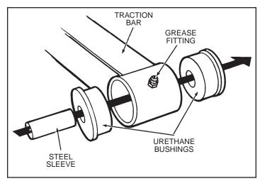
Apply lubricant (supplied) to polyurethane bushings and steel sleeves, then install into eyelet ends as shown.
