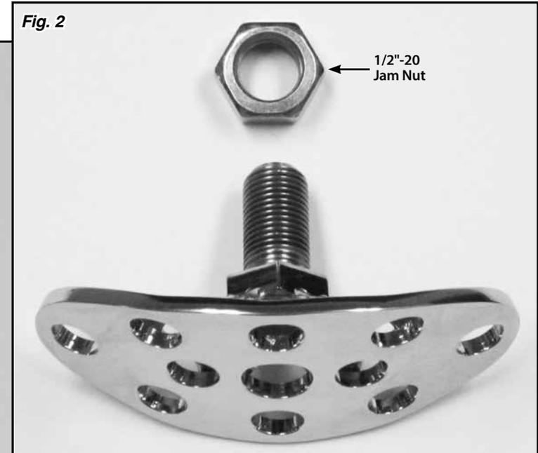
**Step 4: ALL EXCEPT ROUND PEDAL PAD -** Install the 1/2"-20 jam nut onto the threads that protrude beyond the back side of the pedal arm, and tighten the jam nut against the pedal arm. Make sure the Pedal Pad is aligned correctly after tightening.
