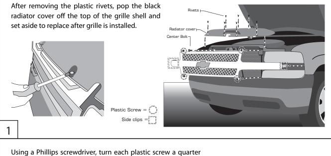
turn to loosen the center of the grille shell.
