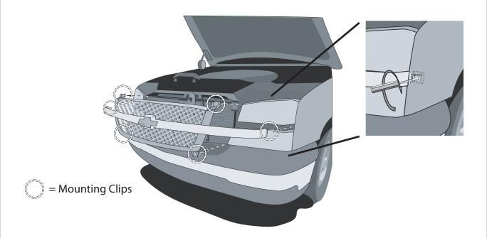
Pull the stock grille shell towards you to remove from the vehicle. Then place the stock grille shell face down. Work on a flat non-abrasive surface such as a blanket or towel to prevent scratching.
