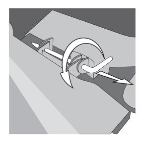
After lights are removed, use a flat head screwdriver to gently pry away the mounting clips that are attached to the mounting brackets on the truck (4 holding the center and one on each side). To get to the side clips, pull the center bar out just enough to slide a flat head screwdriver between the grille shell and the fender. Be extremely careful in between the grille shell and the fender. Touching the side clip, very carefully turn the handle of the screwdriver to pull out the side clip.
