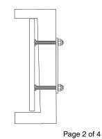
Using a ratchet with a 3/8 socket, tighten each kep nut to a snug fit.
