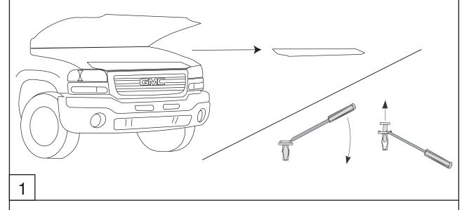
Insert the billet grille over the stock mesh allowing the set screws to go through the stock mesh.
