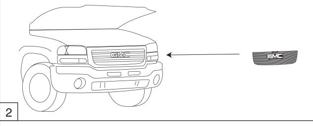
After inserting the billet grille into the vehicle, bolt together using the provided hard-ware.
