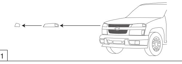
Use a flat head screwdriver to unsnap each clip that holds the stock grille shell to the vehicle. Each arrow indicates approximate location of each clip.
