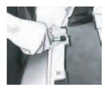
From the back of the bumper, use a Robertson screwdriver to remove the two plastic screws that hold the stock grille to the foam bumper.
