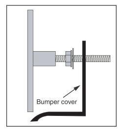
Insert the billet grille into the bumper cover and secure it with a washer and Kep Nut on each mounting stud.
