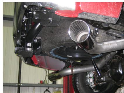
3. Slide a **4"Clamp** onto the lower **Y-Pipe**. Install the **Passenger Side Tail Pipe** from the rear of the truck, over the axle and attach it to the lower section of the **Y-Pipe**. Refer to **Figure 5**.
