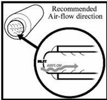
4. Install the **Muffler** over the **Extension Pipe** or over the **Mid Pipe** with 137" wheelbase vehicles. Refer to the figure on the left for correct **Muffler** orientation.
