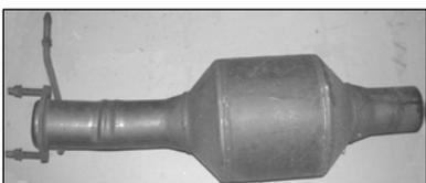
4. Remove the catalytic converter by removing the two nuts holding the inlet flange together using a 15mm wrench or socket. Retain the nuts for the re-installation of the catalytic converter. **See Figure 2.**
