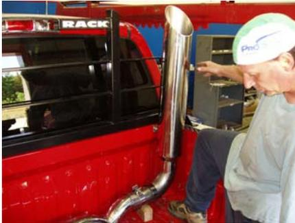
1. Loosely assemble the "T" Pipe assembly in the bed of the truck. Some models may require trimming of the "T" Pipe in order to accommodate the width of the truck bed and the stacks that have been purchased. Be sure to place the **Band Clamps** over the pieces before they are assembled. **See Figure 1.**
