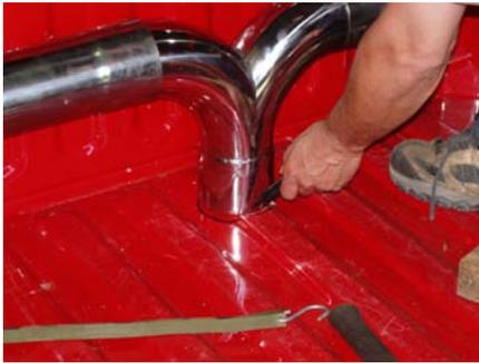
5. Mark the bed floor where the **"T" Pipe** is resting. MBRPinc. recommends tracing around where the **"T" Pipe** meets the bed floor. Remove the stacks, **"T" Pipe**, and **Elbows** from the bed of the truck. Find the center of the circle traced onto the bed floor, mark and center punch it. Make sure that there is clearance for the **Quad Cab Elbow** to pass by any frame cross members. **See Fig 4.**
