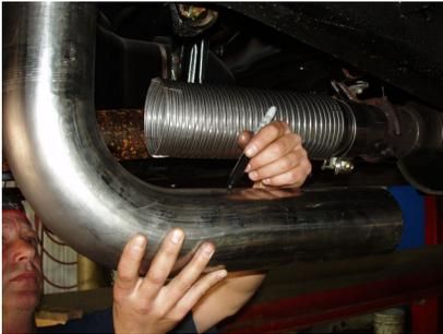
6. Install the **Flexpipe** onto the outlet of the **3.5"-4" Adapter**. Place the **20" Elbow** in position and mark the locations to cut. Allow 3" of overlap at the **Flexpipe** and **20" Elbow** connections. Cut the **20" Elbow** to the required length and install. Remember to slide the required **Band Clamps** onto the parts before assembly. **See Figure 8.**
