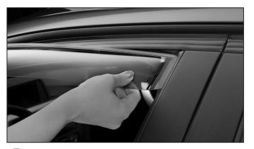
Bow the deflector outward to insert the rear flange into the window channel. Making sure the window gasket is not folded over.
