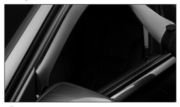
Inspect the deflector to ensure that it is fully inserted into the window channel. Slowly and carefully, close your window fully and press firmly against weather strip from front to rear without engaging auto-up feature.
