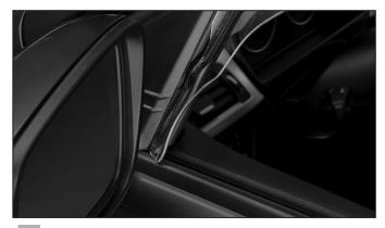
Insert the front of the deflector as shown. Ensure that the edge rests on the top of the outer window sill.
