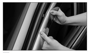
Starting with the front of the deflector, begin tucking the flange into the window channel while pressing inward against the channel clips. Be sure to tuck the flange between weather stripping and the channel clip.
