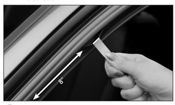
Pull down the weather stripping in the second position, which is approximately 8" from the front mirror.
