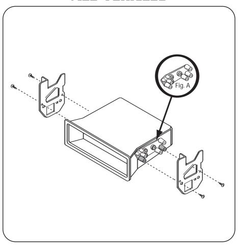
Mount the factory brackets to the *shaded bosses* (Fig A) with (4) #8 x 1/4" Phillip screws supplied and mount the entire assembly to the sub-dash.
