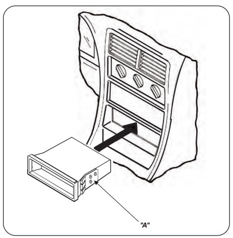
Position the **Pocket** so each Bracket is configured with (2) screws on the top and (1) screw on the bottom ("A"). Slide the **Pocket** into the dash opening until the side clips engage.
