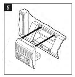
Re-connect the battery terminal and test the unit for proper operation. Snap the head unit/trim bezel assembly into the sub-dash.
