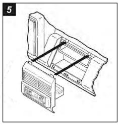
Re-connect the battery terminal and test the unit for proper operation. Snap the head unit/trim bezel assembly into the sub-dash.
