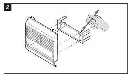
Using the *Radio Housing* as a template, carefully scribe the radio opening onto the back of the radio trim bezel. Cut the bezel along the scribed lines and remove the trimmed portions. (If a factory pocket is molded into the bezel, cut and remove the pocket as well).
