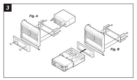
**2-SHAFT HEAD UNITS:** Align the radio opening in the **Radio Housing** with the radio opening in the radio trim bezel and mount the Housing to the back of the bezel with **(4) Phillips Panhead Screws** supplied. Place the desired **Faceplate** against the front of the bezel. Slide the aftermarket head unit through the assembly and secure with shaft nuts. (see Fig. A)
