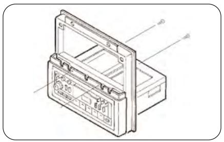
Secure the radio housing to the support plate with (2) hex-head screws previously removed on page 1.
