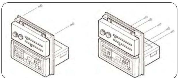
Mount the climate control cluster to the front of the support plate with (2) hex-head screws previously removed on page 1
