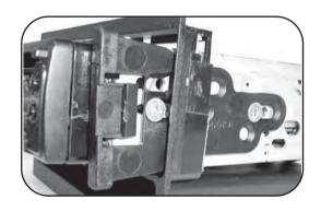
**NOTE:** When reinstalling the screws into the bottom of the 99-5806 use the (2) supplied Phillips screws instead of the factory screws removed in step **5** in Dash Disassembly.
