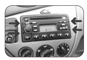
1 Using Metra's 86-5618, pull the factory head unit from the dash and disconnect the wiring.
