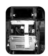
9 Remove the (4) Phillips screws securing the factory climate control button assembly to the radio panel and remove. Note: Retain all hardware to be used in Kit Assembly. (Figure H)
