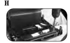
10 Remove (4) Phillips screws securing the factory pocket assembly to the radio panel and remove. Note: Retain all hardware to be used in Kit Assembly. (Figure 1)
