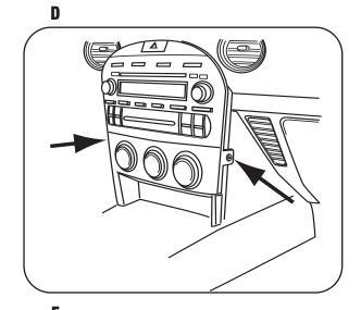
Pull radio/climate control panel out, disconnect plugs and remove. (Figure E)
