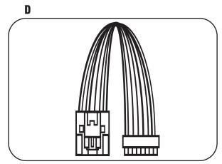
NOTE: This 16 to 16 position harness is <u>NOT USED</u> with <u>ELECTRONIC</u> CLIMATE CONTROL vehicles.
