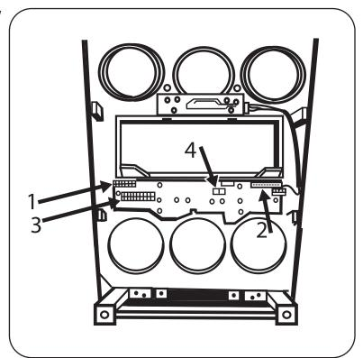
**Note:** The connector "2" is not used in this application.
