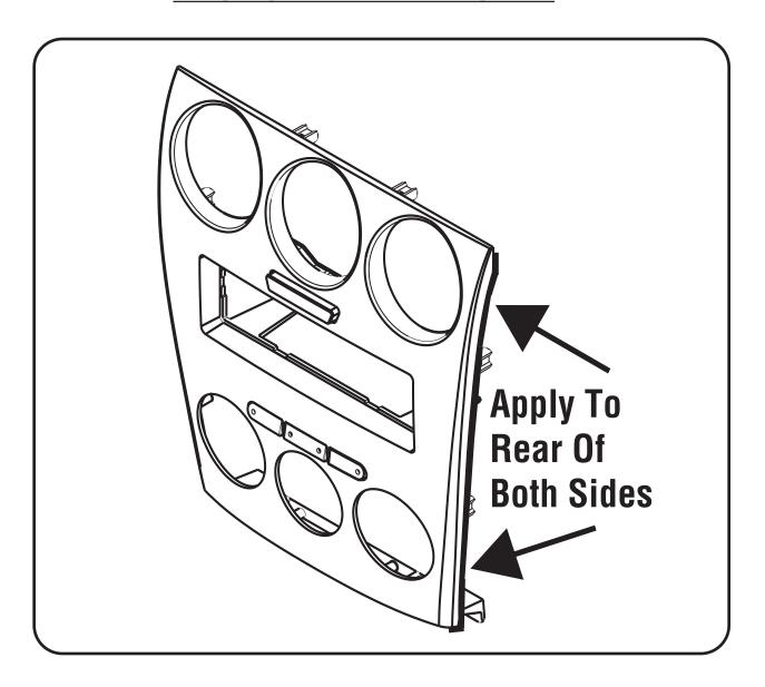
**Note:** Due to differences in factory tolerances you may need to apply the provided felt tape to the edge of the 99-7507 radio housing to relieve backlight bleed through.
