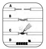
(A) Strip wire ends back 1/2" B) Twist ends together C) Solder D) Tape
