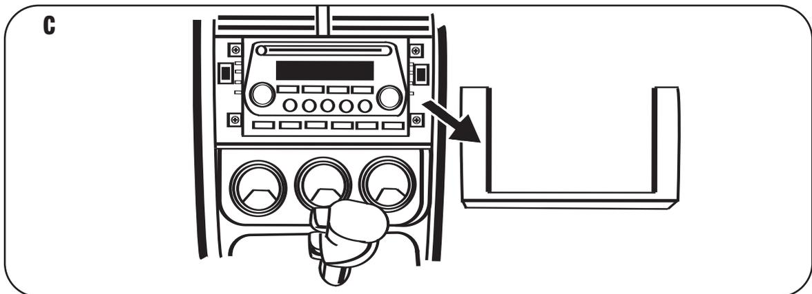
**NOTE:** As an option, the center panel (the smaller piece around radio) is all that needs to be removed, but it is very prone to damage, so full panel removal is recommended. (Figure C)
